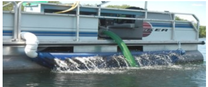
A Marinette County DASH unit sucks in milfoil and water (green tube) and discharges water from another tube.
